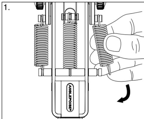
Attach two outer springs to the lamp, stretching slightly as necessary.
