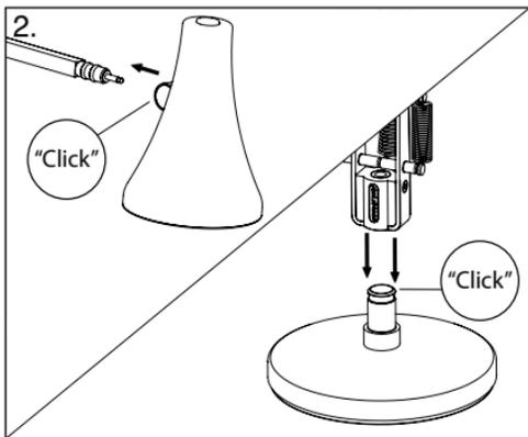
With base on flat surface, attach arm and shade to connectors. Press down to engage.
