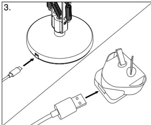
Connect one end of cable to USB port on lamp base, the other to plug adaptor.
