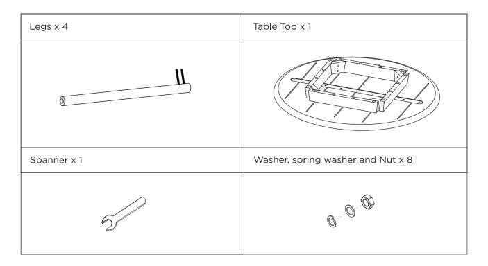
Always assemble table on a soft clean surface. Use spanner provided to tighten all nuts. Always use two people to flip the table over to an upright position. Match each numbered leg to the corresponding numbered corner.
