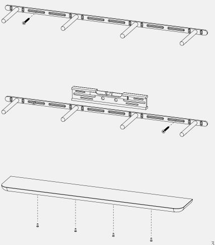
Locate bracket at desired wall position on wall, screw in first screw.
