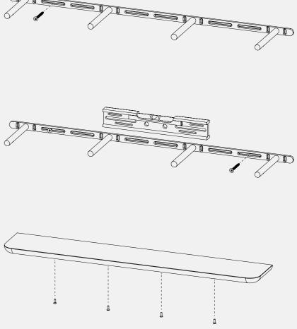
Level the bracket using a spirit level and screw in the second screw followed by the remaining screws.
