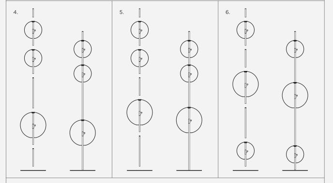
parts used: top stem + small shade  $\times$  2 + large shade + short extension pole + long extension pole + base. parts spare: short extension pole  $\times$  1
