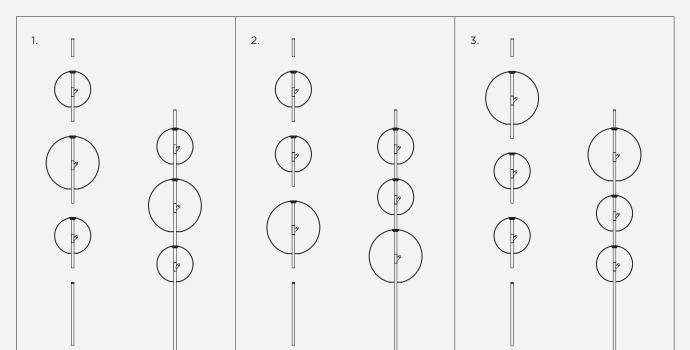
parts used: top stem + small shade  $\times$  2 + large shade + long extension pole + base. parts spare: short extension pole  $\times$  2
