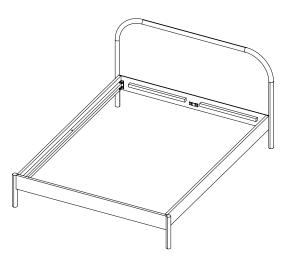
Attach legs to centre brace using M8 screws and allen key provided. Locate centre brace by slotting into the pre-fitted brackets on headboard and footboard. Adjust feet on legs if needed.
