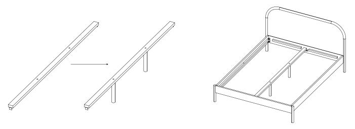
Secure cross brace using M6 screws, washer and spring washer with allen key provided. Tighten all nuts evenly to secure. Lower slats gently into place to complete assembly.
