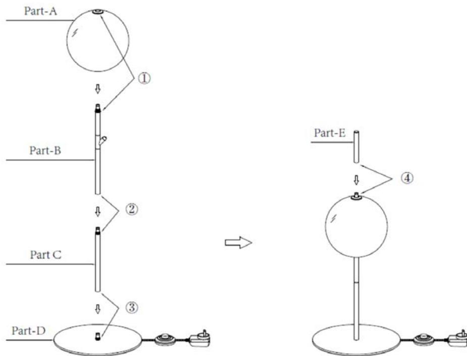
1. The lampshade and stem are connected by threads.
