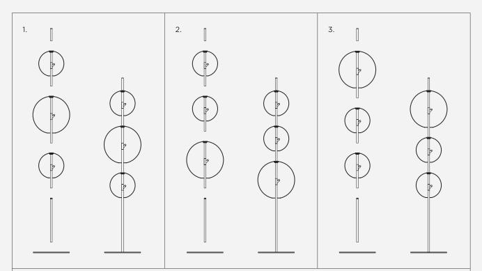
parts used: top stem + small shade  $\times$  2 + large shade + long extension pole + base. parts spare: short extension pole  $\times$  2
