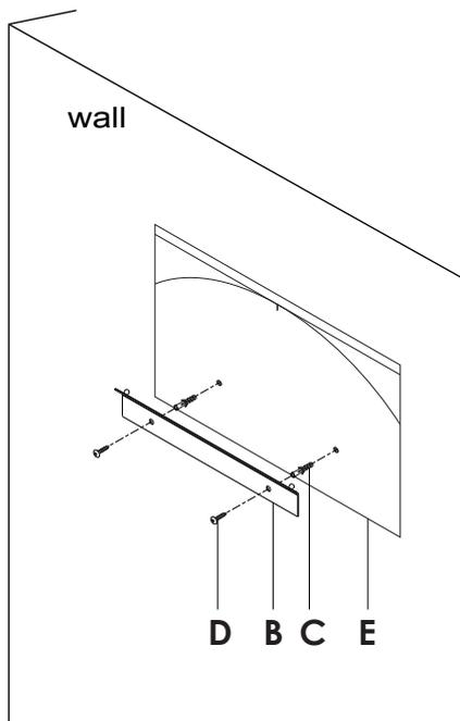
1. Attach the drilling template (part E) to the wall, with the curved line representing the top of the mirror. drill holes into the two marks indicated on the drilling template. remove the template and screw the bracket (part B) into the wall.
