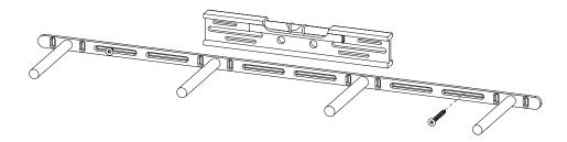
3. Locate the shelf on the wall bracket, secure shelf with bolts.
