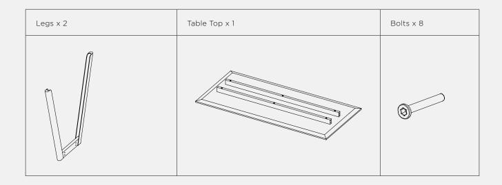
Place tabletop upside down on a clean soft surface. Locate the legs onto the tabletop. Using the hex key provided; tighten each bolt through the leg hole into the tabletop rail. Once the legs are secured, use two people to flip the table into the upright position.
