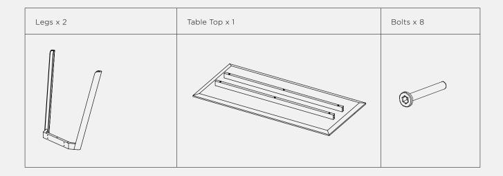
Place tabletop upside down on a clean soft surface. Locate the legs onto the tabletop. Using the hex key provided; tighten each bolt through the leg hole into the tabletop rail. Once the legs are secured, use two people to flip the table into the upright position.
