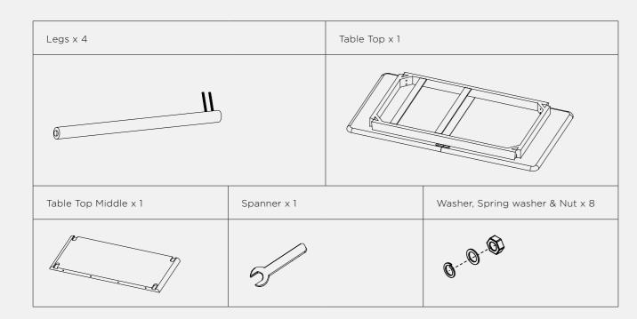
Assemble table on a soft clean surface. Use spanner provided to tighten all nuts. Always use two people to flip the table over to an upright position. Match each numbered leg to th corresponding numbered corner.
