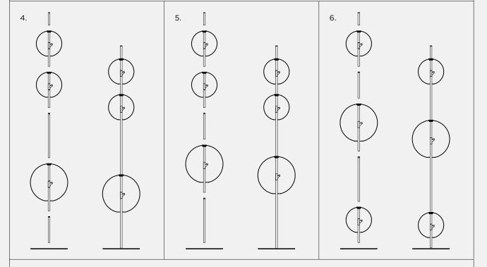
Parts Used: Top stem + small shade x 2 + large shade + short extension pole + long extension pole + base.
