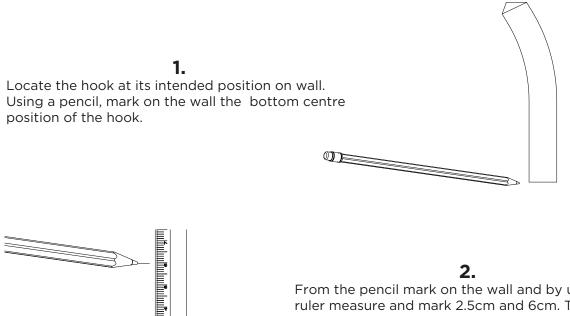
From the pencil mark on the wall and by using a ruler measure and mark 2.5cm and 6cm. This will provide you with the two fixing points for the screws. Double check that distance between the two screw holes marks are 3.5cm. *hint\* to make sure your hook hangs perfectly straight; you can use a level or a level phone app to make sure the two screw hole marks are vertical.*
