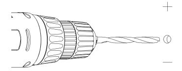
**3.** Using a drill and 5mm drill bit, drill two holes into the two screw hole marks on the wall.
